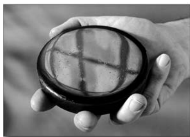
Test glass produced by vitrification process.
