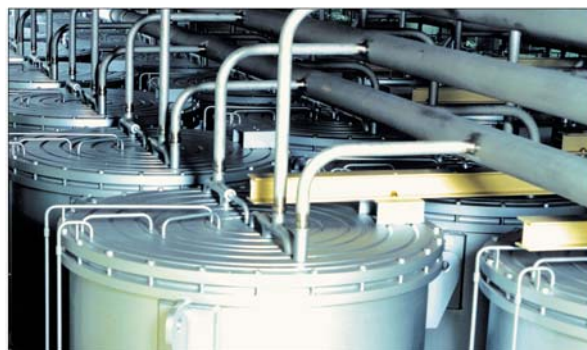
Cascade of centrifuges at Rokkasho-mura in Japan.
